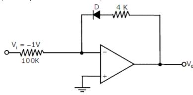
For an input voltage  $V_1 = -1V$ , the output voltage  $V_0$  is
