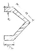
IX. A section which is subjected to twisting is shown below. Determine the allowable twisting moment for a maximum shear stress of 68 950 k Pa. Calculate the shear stresses in different parts of section neglecting stress concentration.
