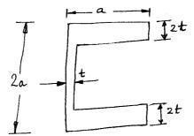
IX. A thin-walled box shown in figure is subjected to a torque T. Determine the shear stresses in the walls and the angle of twist per unit length of the box. (20)
