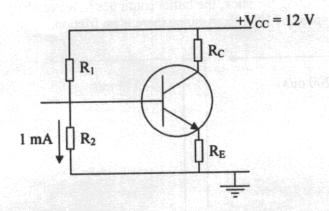
Given that  $V_E$  = 2 V,  $V_{BE}$  = 0.6 V and  $I_C$   $\cong$   $I_E$ , find the values needed for the resistances  $R_1$ ,  $R_2$ ,  $R_E$  and  $R_C$ . (15)
