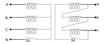
The star-delta transformer shown above is excited on the star side with a balanced, 4-wire, 3-phase, sinusoidal voltage supply of rated magnitude. The transformer is under no load condition.
