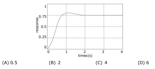
28. The open loop transfer function of a unity feedback system is given by  $G(s) = (e^{-0.1s})/s$ . The gain margin of this system is
