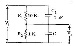
A RC potentiometer to measure ac voltage, it is desired that  $\frac{V_{o}}{V_{i}}$  should be independent of
