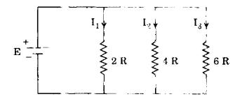
Three parallel branches of resistors are connected across a dc source as shown in the figure. What is  $I_1$ :  $I_2$ :  $I_3$ ?
