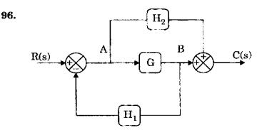
The transfer function  $\frac{C(s)}{R(s)}$  for the system
