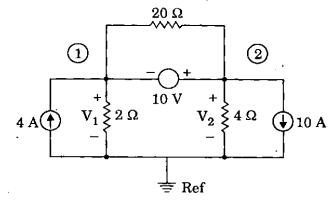
When KCL is applied at the super node in the above circuit, the current equation in terms of node voltages  $V_1$  and  $V_2$  is
