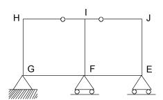
Q.33 The members EJ and IJ of a steel truss shown in the figure below are subjected to a temperature rise of 30°C. The coefficient of thermal expansion of steel is 0.000012 per °C per unit length. The displacement (mm) of joint E relative to joint H along the direction HE of truss, is
