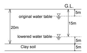
Q.80 What is the change in the effective stress in  $kN/m^2$  at mid-depth of the clay layer due to the lowering of the water table?
