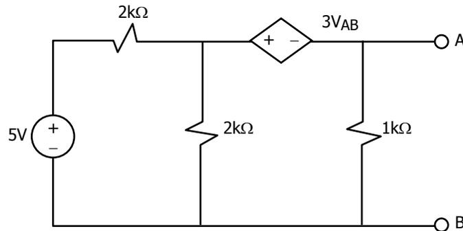
59. For the circuit given above, the Thevenin's resistance across the terminals A and B is
