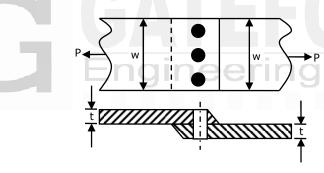
Width of the plate w=200 mm, thickness of the plate t=5 mm, number of rivets n=3, diameter of the rivet  $d_r = 10 \, \text{mm}$ , diameter of the rivet hole  $d_h = 11 \, \text{mm}$ , allowable tensile stress of the plate  $\sigma_p$  = 200 MPa, allowable shear stress of the rivet  $\sigma_s$  = 100 MPa and allowable bearing stress of the  $\sigma_c$  = 150 MPa
