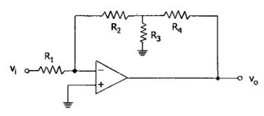
(c) Derive an expression for the closed loop gain  $v_0/v_i$  of the circuit shown above. Assume ideal OP AMP. 10 Using J-K flip-flop, design a counter which has the following count sequence:
