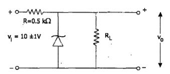
A Zener regulator circuit is shown above in which the nominal supply voltage is 10 V but can vary by  $\pm$  1V. The ratings of Zener are;  $V_Z = 6.8$  V,  $I_z = 5$  mA,  $r_z = 20$   $\Omega$  and  $I_{zk} = 0.2$  mA. Determine
