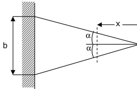
52. The area moment of inertia about the neutral axis of a cross-section at a distance  $x$  measured from the free end is
