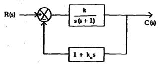
Determine the value of k and velocity feedback constant  $k_v$  so that the maximum overshoot in the unit step response is 0.2 and the peak time is 1 sec. With these values of k and  $k_v$ , obtain the rise time and settling time.
