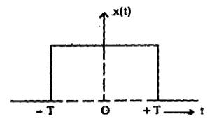
For the rectangular pulse shown in the above figure, determine the Fourier Transform of x(t) and sketch the magnitude spectrum with respect to frequency.
