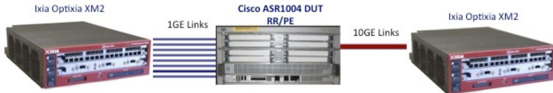
Figure 1: Cisco ASR 1004 Control Plane and provider-edge testing
