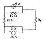
In the circuit shown in the given figure, RL will absorb maximum power when its value is
