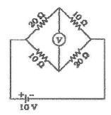
The reading of high impedance voltmeter V in the bridge circuit shown in the given figure is
