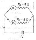
Here,  $R_1$  and  $R_2$  are in parallel
