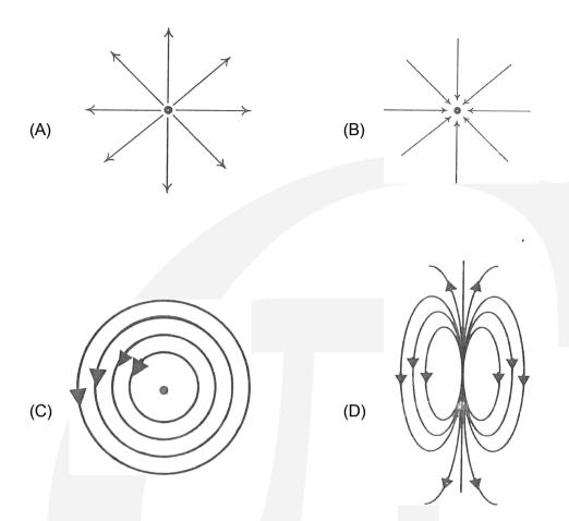
27. **(C)** Electric field produced by the time varying magnetic field is circular. For a long straight wire, the magnetic field lines are circles with their centres on the wire.
