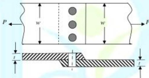
width of the plate  $w = 200 \text{ mm}$ , thickness of the plate  $t = 5 \text{ mm}$ , number of rivets  $n = 3$ , diameter of the rivet  $d_r = 10 \text{ mm}$ , diameter of the rivet hole  $d_h = 11 \text{ mm}$ , allowable tensile stress of the plate  $\sigma_t = 200 \text{ MPa}$ , allowable shear stress of the rivet  $\sigma_s = 100 \text{ MPa}$  and allowable bearing stress of the rivet  $\sigma_c = 150 \text{ MPa}$ .
