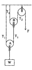
Neglecting the friction and weights of the pulley, which one of the following is the force 'F' required to lift a 100 N load in the system of pulleys as shown in the above figure?
