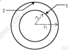
The view factor  $F_{21}$  for radiation heat transfer is
