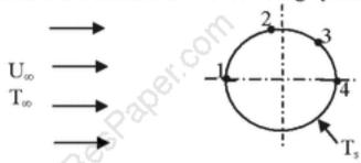
The free stream velocity is  $U_{\infty}$  and the free stream temperature  $T_{\infty}$  is lower than the cylinder surface temperature  $T_s$ . The local heat transfer coefficient is minimum at point
