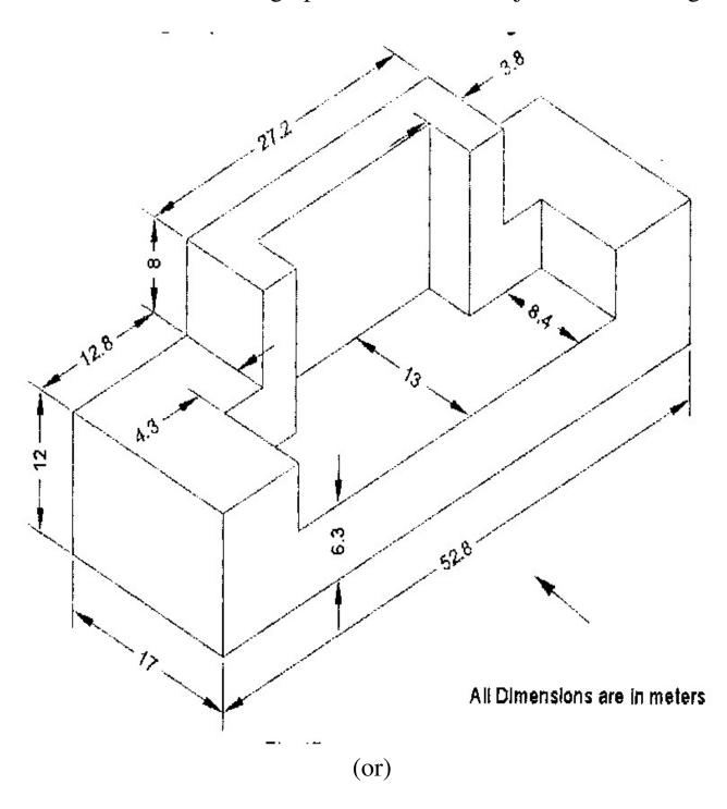
20. Draw the front view, top view and right side view of the object shown in fig.2.
