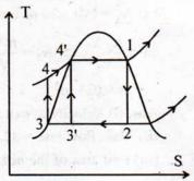
(iii) Vapour has large specific volume. So size of compressor (pump) becomes large in Carnot cycle. More power is required; so plant efficiency is low.
