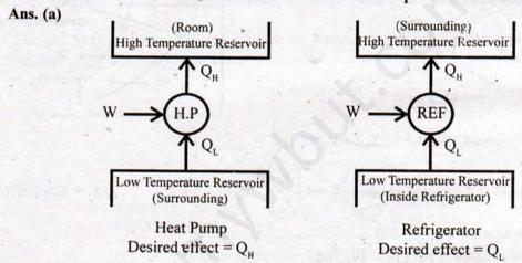
A refrigerator is a device which, operating in a cycle, maintains a body at a temperature lower than the temperature of the surroundings. On the other hand, a heat pump is a device which, operating in a cycle, maintains a body at a temperature higher than the temperature of the surrounding.
