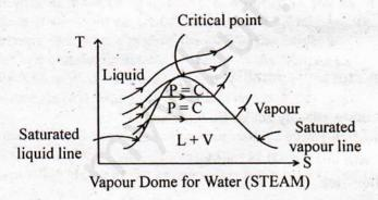
represent the critical point on a T-S plane at which there is no transition zone from liquid to vapour. The temperature, pressure and volume of water at critical point are called critical temperature, critical pressure and critical volume.
