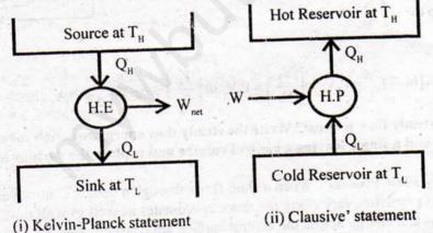
Ans. (b) A perpetual motion machine of 2nd kind or PMM2 is a fictitious heat engine that will produce network in a complete cycle by exchanging heat with only one reservoir, thus violating the Kelvin Planck statement.
