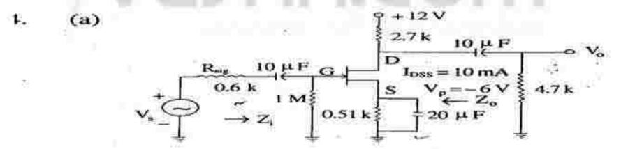
For the above JFET  $I_{DSS} = 10 \text{ mA}$  and  $V_p = -6 \text{ V}$ .
