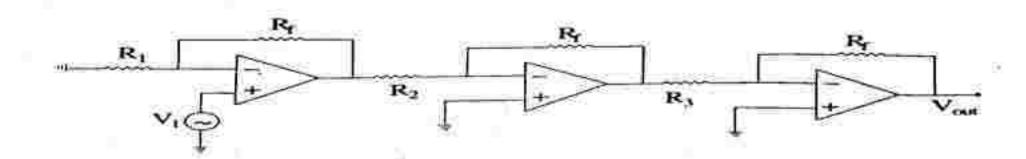
If  $V_1 = 50 \mu v$ ,  $R_1 = 4.7 k$ ,  $R_2 = 47 k$ ,  $R_3 = 47 k$  and  $R_r = 470 k$ , find the overall gain of the amplifier.
