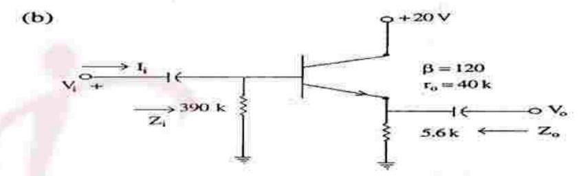
Draw the a.c. equivalent circuit. Determine  $Z_i$ ,  $Z_o$ ,  $A_v$  and  $A_v$ .
