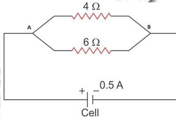
ii. In parallel combination of resistors potential difference across each resistor is same as the potential difference across the terminals of the battery.
