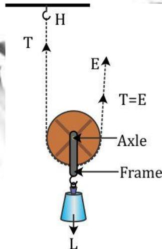
The load  $L$  is balanced by the tension in two segments of the string and the effort  $E$  balances the tension  $T$  at the free end, so
