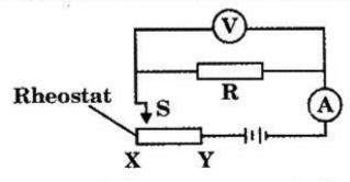
The reading of the ammeter is I and that of the voltmeter is V. How do the values of I and V change when the sliding contacts of the rheostat are slowly moved from X to Y?
