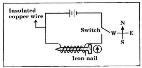
What will you observe in the compass shown in the above figure when the circuit is switched on?
