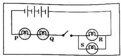
Identify the bulbs that glow when switch is in the 'OFF' position?
