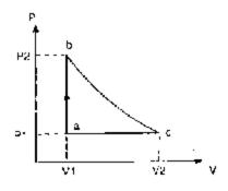
shown in the figure. The gas absorbs 7000 J of heat as its temperature increases from 300 K to 1000 K, in giving from a to b. The quantity of the heat rejected by the gas during the process ca-
