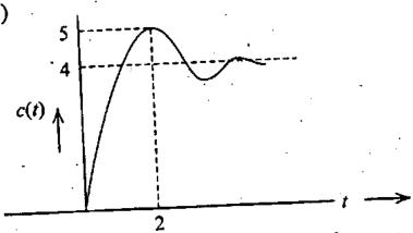
The step response of second order system is shown in the above figure for an input of 4 u(t). Determine the open loop and closed loop transfer function. Assume unity feedback.
