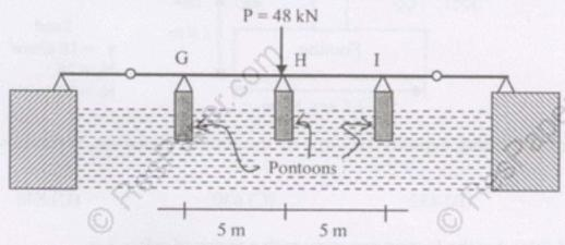
Q.76 When the middle pontoon is removed, the deflection at H will be
