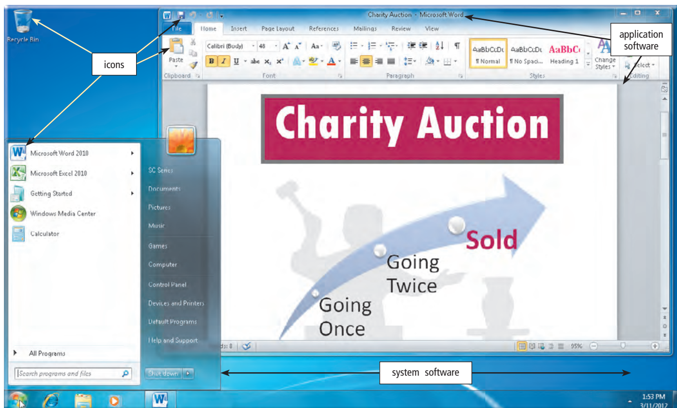
Figure 1-10 Today's system software and application software usually have a graphical user interface.
