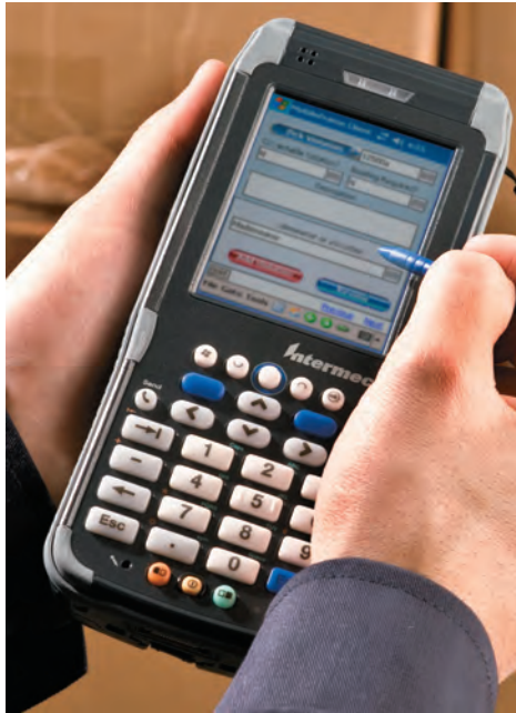
Figure 1-21 This handheld computer is a lightweight computer that enables delivery people to obtain and record information about their deliveries.
