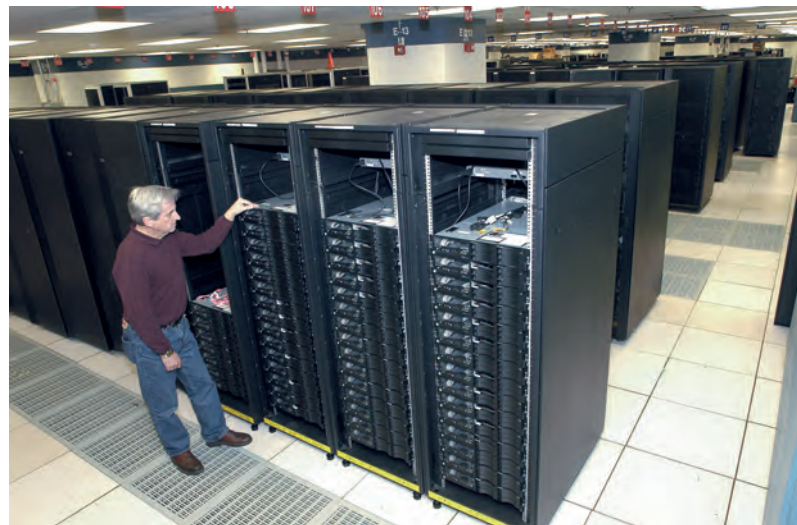
Figure 1-27 This supercomputer, IBM's Roadrunner, can process more than one quadrillion instructions in a single second.
