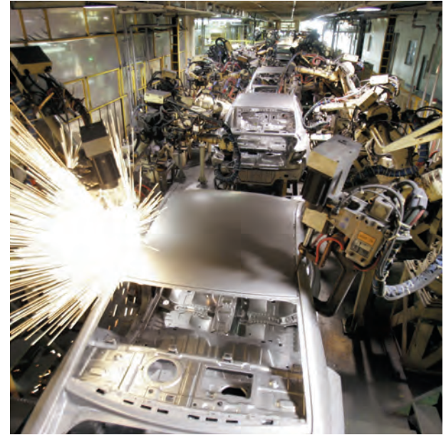
Figure 1-43 Automotive factories use industrial robots to weld car bodies.
