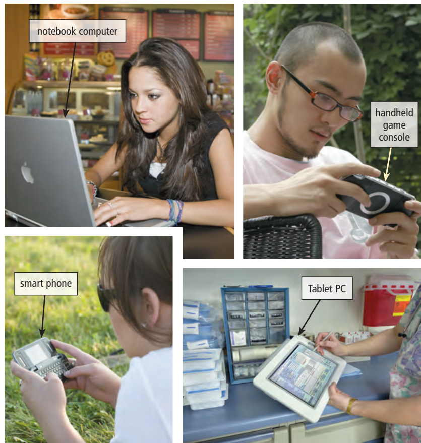
Figure 1-32 Mobile users have a variety of mobile computers and devices so that they can work, do homework, send messages, connect to the Internet, or play games while away from a wired connection.
