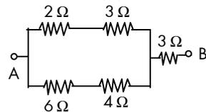
In the above circuit, the effective resistance between the points A and B is
