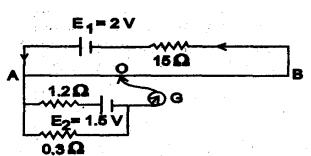
Calculate (i) potential gradient along AB, and (ii) length AO of the wire, when the galvanometer shows no deflection.
