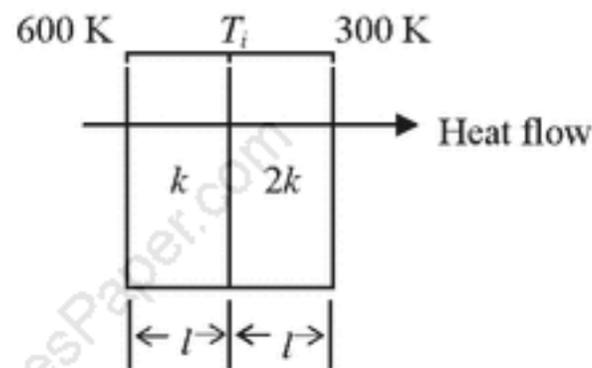
The interface temperature  $T_i$  (in K) of the composite wall is \_\_\_\_\_
