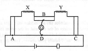
The figure shows experimental set up of a meter bridge. When the two unknown resistances X and Y are inserted, the null point D is obtained 40 cm from the end A. When a resistance of 10  $\Omega$  is connected in series with X, the null point shifts by 10 cm. Find the position of the null point when the 10  $\Omega$  resistance is instead connected in series with resistance 'Y'. Determine the values of the resistances X and Y.
