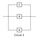
Suppose that each of the three components fail with probability p and independently of each other. Let  $q_i$  = Prob (Circuit i does not fail); i = 1,2,3. For 0 , we have
