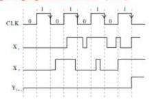
This is a synchronous circuit, so both the flip flops will trigger at the same time and will respond on falling edge of the Clock. So, the correct output (Y) waveform is associated to w<sub>3</sub> waveform.
