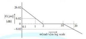
If the system is connected in a unity negative feedback configuration, the steady state error of the closed loop system, to a unit ramp input, is \_\_\_\_\_\_.
