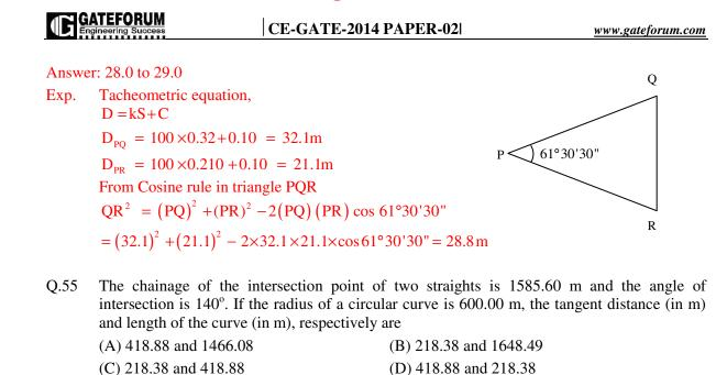
Answer: (C) Exp. Length of curve,  $L = \frac{\pi}{180} \times \Delta \times R$   $= \frac{\pi}{180} \times 40 \times 600 = 418.88m$ Tangent distance,  $T = R \tan\left(\frac{\Delta}{2}\right)$  $= 600 \tan\left(\frac{40}{2}\right) = 218.38m$ R  $\Delta^{2} \Delta^{2}$ R
