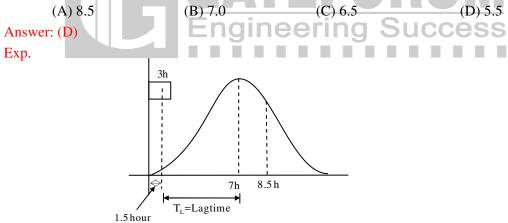
For small catchment, time of concentration is equal to lag time of peak flow.  $T_c = 7 - 1.5 = 5.5 \text{ h}$
