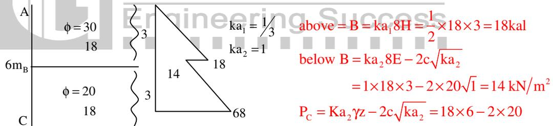
$$P_a = \frac{1}{2} \times 18 \times 3 + \frac{1}{2} (14 + 68) \times 3 = 150 \text{ kN/m}^2$$
