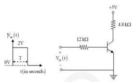
For the inputV<sub>in</sub>(t) as shown in the figure, the transistor switches between the cut-off and saturation regions of operation, when T is large. Assume collector-to-emitter voltage saturation  $V_{CE(sat)}$ =0.2V and base-to-emitter voltage  $V_{BE}$ =0.7V. The minimum value of the common-base current gain (a) of the transistor for the switching should be
