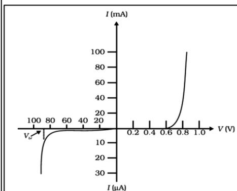
The direction of the applied voltage (V) is opposite to the built-in potential  $V_0$  in the semiconductor diode. As a result, the width of depletion layer decreases and the barrier height is reduced.
