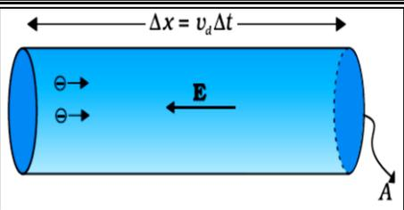
Drift velocity:  $\vec{v}_d = \left(-\frac{e\vec{E}}{m}\right)\tau$  and  $|\vec{v}_d| = \frac{e|\vec{E}|\tau}{m}$  .....(1)
