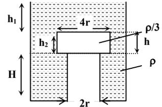
24. If level of liquid starts decreasing slowly when the level of liquid is at a height  $h_1$  above the cylinder, the block just starts moving up. Then, value of  $h_1$  is
