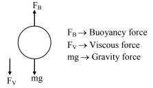
Buoyancy force is due to pressure difference.
