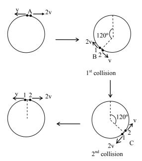
First collision will occur at point 'B' as shown in figure. Velocity of balls 1 and 2 will get inter-changed and second collision will occur at point 'C'. Again the velocity of balls 1 and 2 will get inter-changed and the two balls will collide again at 'A'.
