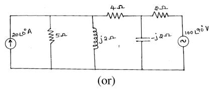
12. Calculate the current through the  $5\Omega$  using Thevenin's theorem.
