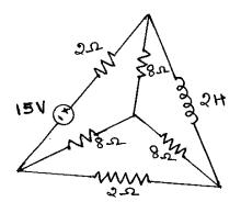
19. The switch in circuit was open for a very long time, but closed at t = 0. If i(0) = 10A, find i(t) for t > 0 by Pspice.
