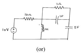
18. Write the fundamental tie set matrix and cur set matrix for the network shown.
