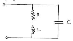
17. Draw the dual circuit for the given network and give the element values.
