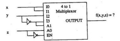
The function f(x, y, z) implemented by the above circuit is
