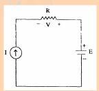
For the circuit shown, what is the voltage V if the source voltage is reduced by 50%?
