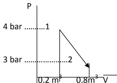
vii) Calculate the heat transferred during the cycle shown in the figure given below.
