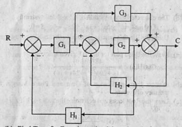
(b) Find Transfer Function using Mason's gain formula: 10
