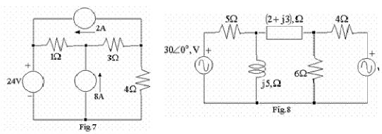
b. Find  $v_x$  in the network of Fig.8, if the current through (2 + j3) element is zero. (8)
