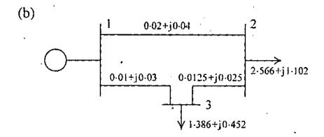
The one-line diagram of a simple three-bus power system with generator at bus 1 is given above. The line impedances are marked in per unit on 100 MVA base. The voltages obtained by performing load flow are:
