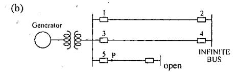
The single-line diagram of a three-phase power system is given above. The generator is delivering 1.0 per unit power to the infinite bus. The pre-fault power angle equation is
