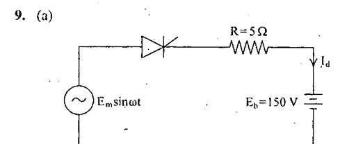
A dc battery is charged through a resistor R as shown in the above figure. Derive an expression for the average value of charging current in terms of  $E_m$ ,  $E_b$ , R. Assume that the SCR is fired in every cycle.
